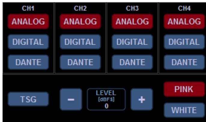
The Channel Source frame allows to select the source type of each input channel (ANALOG, DIGITAL or DANTE), or to enable the internal test signal generator (TSG). The current source selection is shown with red buttons.
